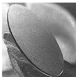
A magnified image of an Artificial Silicon Retina chip.
